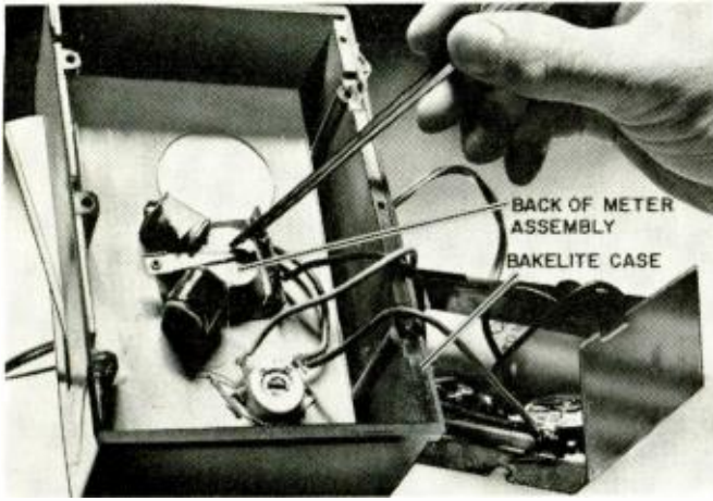
Fig. 8—Back of meter assembly (manual type).
